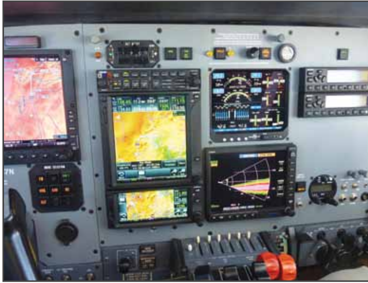
This closeup of the center stack shows the new logical layout and uncluttered look of my new panel. Note the lighted Eaton switches and their strategic locations.
