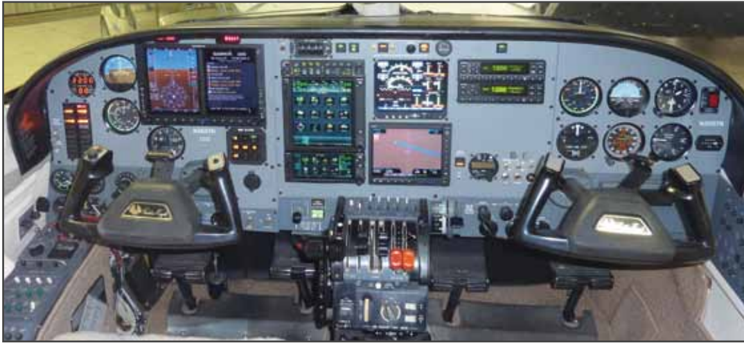
Everything communicates! Tying everything together in a way that ensures easy and seamless operation is a tribute to both Garmin engineering and my installer, Executive Aircraft Maintenance of Scottsdale. The logical layout was the result of 10 different CAD revisions!
